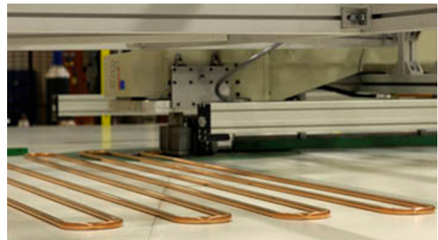
Picture 2: Atrium Plana high precision laser welding.
