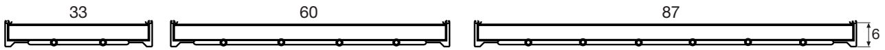
Figure 2. Atrium and Loggia are manufactured as standard in three widths, 33, 60* and 87 cm, and one height, 6 cm. Actual width dimension is -8 mm.
