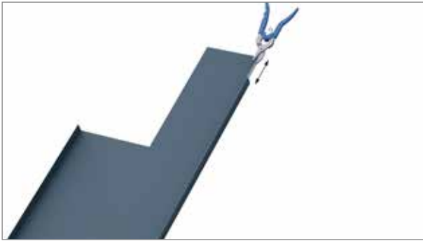
Cut off the part of the joint that goes in the overlap.
