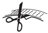
B. "Dial up" the required clip diameter aligning the armwith the radial dimensioned markings on the case and cut to length at the cutting indicator mark.
