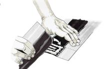
Coat the cloth with the appropriate adhesive or use our self-adhesive pads (if appropriate). Join both sides and press together firmly
