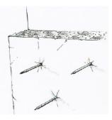
Insulation can be impaled immediately but maximum strength of adherence is achieved after 24 hours.
